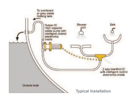
**Unique Intelligent Control means that** Grey IC Kit is all you need to manage waste from multiple drains through one pump
